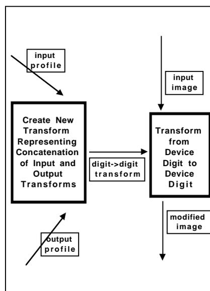
Figure 1c: Typical ICC image processing with efficiencies. Transform box may include 1-D and 3-D lookups and matrices.
