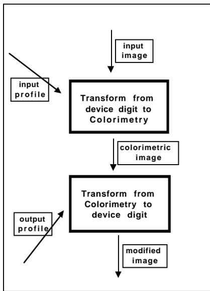
Figure 1b: Logical ICC image processing block diagram.
