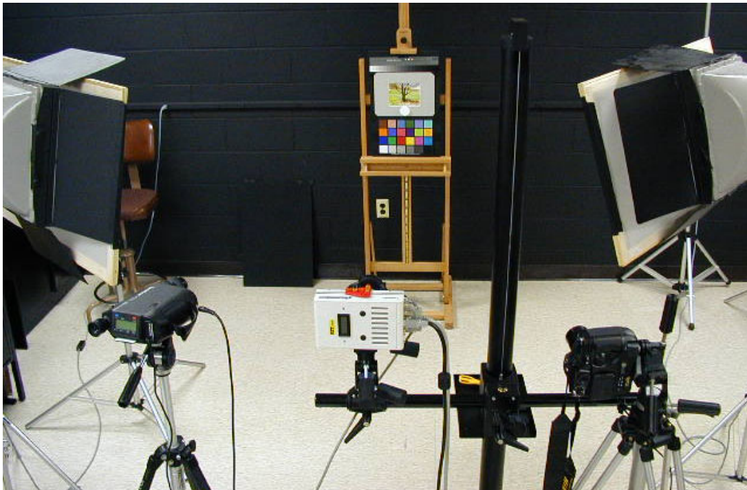
Figure 1. Phase I imaging system. A PhotoResearch PR650 is shown on the left. It is used to make direct measurement of the lighting system. In the center is the Quantix sensor. On the right is the Nikon D-1 digital camera, used to provide a benchmark.
