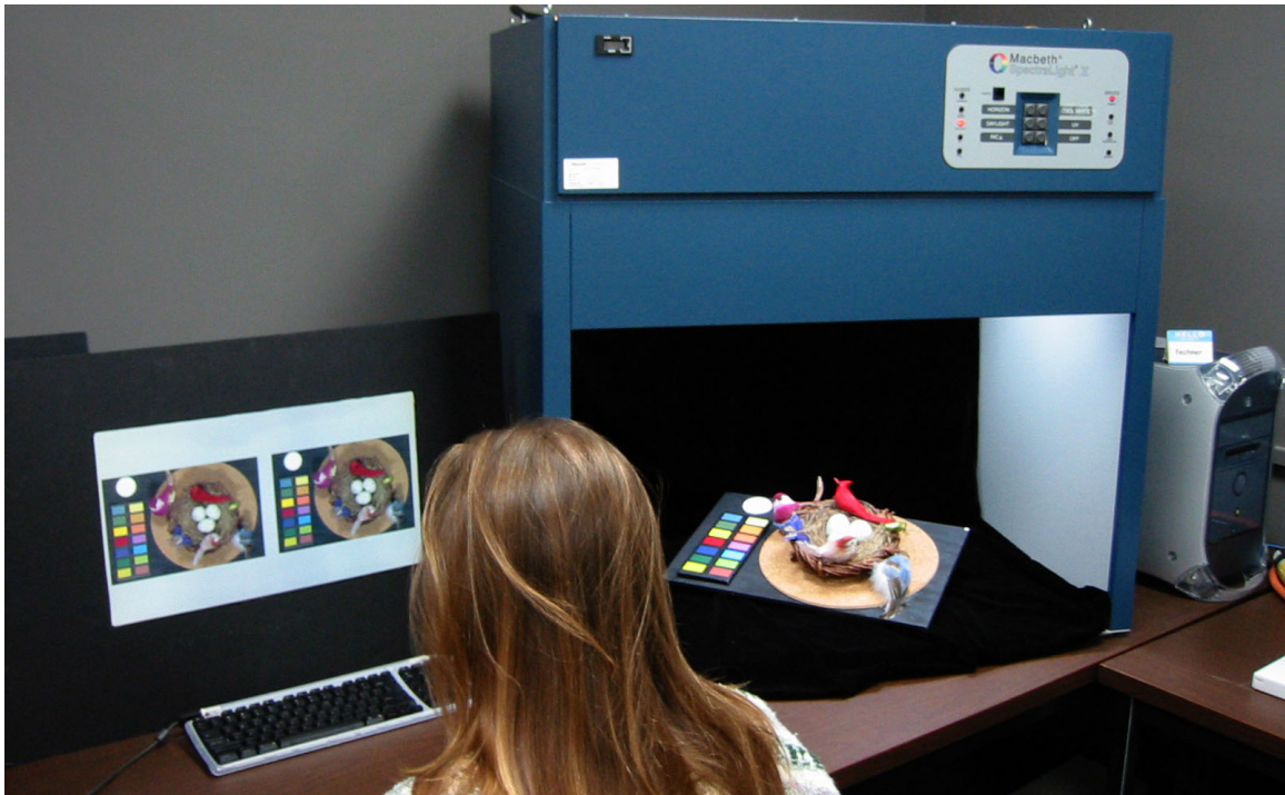
Figure 2. Viewing environment for evaluating color and spatial image quality. Image pairs are shown on an Apple Cinema Display via the Matlab software environment. Various test targets are placed in the Macbeth light booth.
