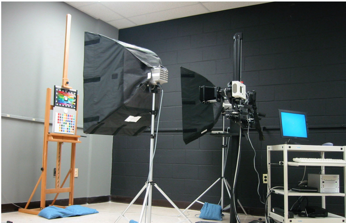
Figure 6. Phase I updated imaging system. On the easel is the GretagMacbeth ColorCheckerDC, used to calibrate the imaging system. Below it is an oil-paint target.
