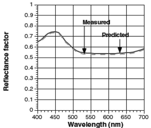
Figure 2c. Light blue mismatch with 0.01 shift in amplitude.
