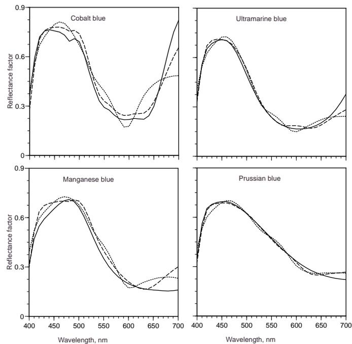
Figure 3. Spectral estimation of four samples from the paint target: measured (solid line), estimated from spectral data of ColorChecker (dotted line), estimated from spectral data of the entire target (dashed line)
