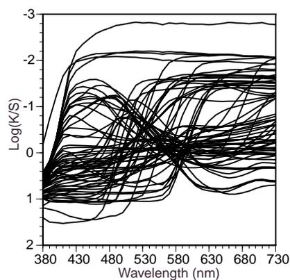
Figure 2.  $\text{Log}(K/S)$  spectra of the 68-pigment paint target
