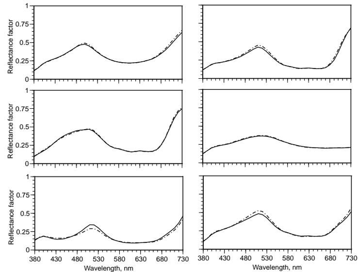
Figure 1. Measured (solid lines) and estimated (dot-dashed lines) spectra of six unknown two-chromatic pigment mixtures using the Berns method (Berns et al. 2002)
