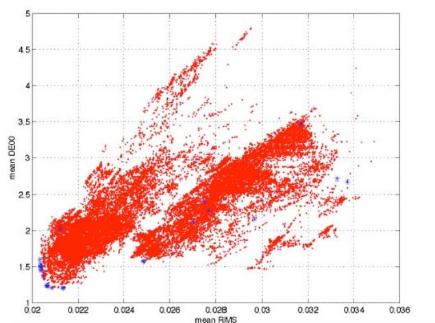
Figure 2. Mean color differences ( $\Delta E_{00}$  for D65) compared with spectral error, RMS, in the estimation of the Esser calibration target for the selected 30,000 filter pairs. Blue asterisks mark 25 filter pairs selected for further analysis.
