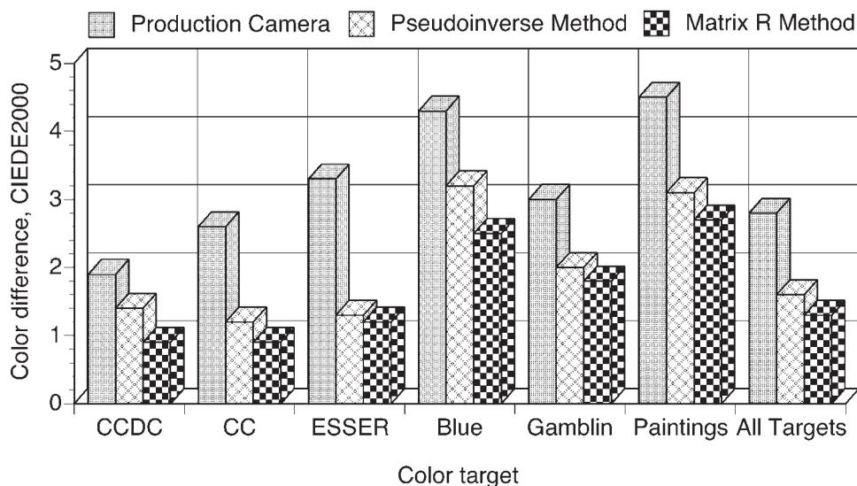
FIG. 2. Comparison of average CIEDE2000 color difference between one colorimetric method of the production camera and two spectral reconstruction methods for the modified camera.
