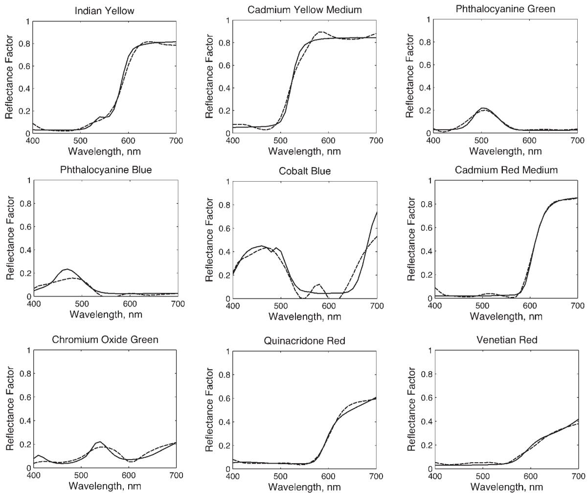
FIG. 5. Measured (solid line) and predicted (dashed line) spectral reflectance factors using the matrix R method. 1: Indian Yellow 2: Cadmium Yellow Medium 3: Phthalocyanine Green 4: Phthalocyanine Blue 5: Cobalt Blue 6: Cadmium Red Medium 7: Chromium Oxide Green 8: Quinacridone Red 9: Venetian Red.
