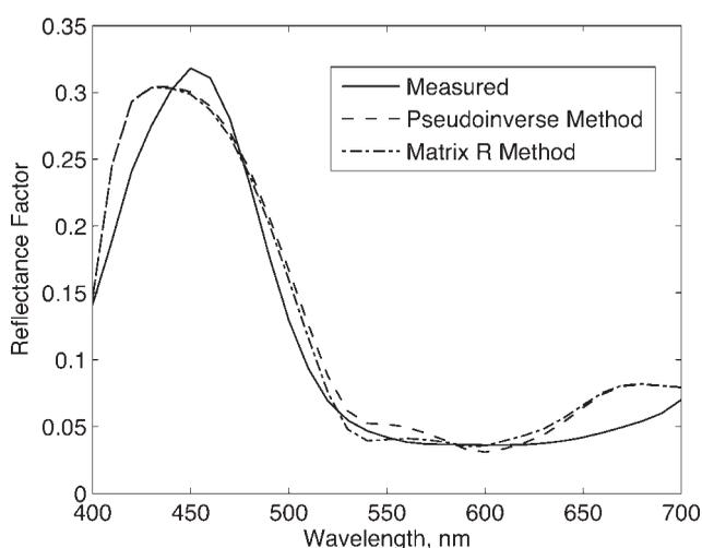
FIG. 3. Comparison of measured reflectance factor (solid line) with predicted ones from the pseudoinverse method (dashed line) and matrix R method (dash-dotted line). The color differences between measured and predicted reflectance factors from the pseudoinverse and matrix R methods are 3.2 and 0.8, respectively.
