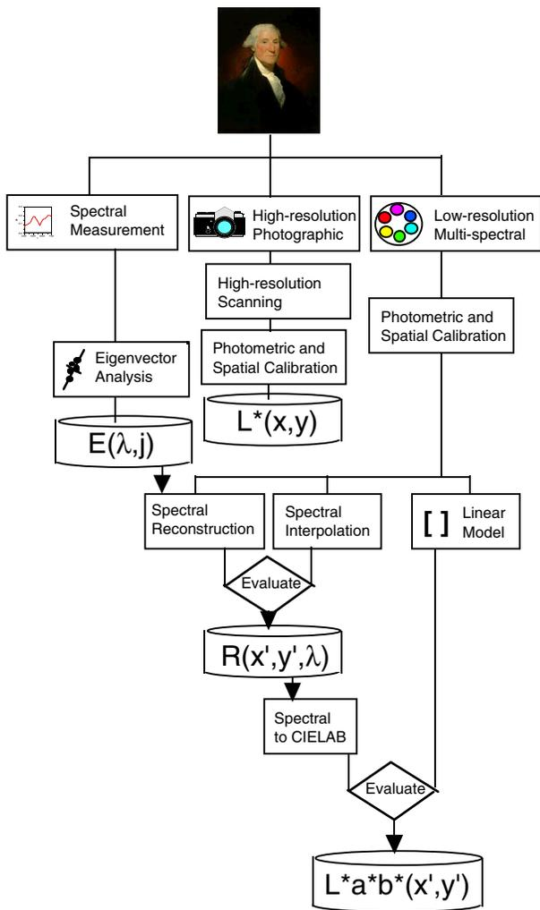
Figure 1. Image acquisition and spectral analysis flowchart
