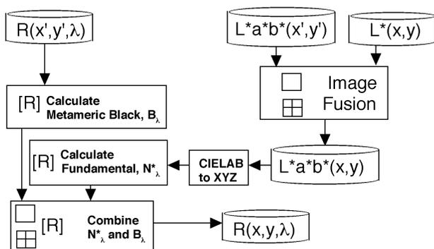
Figure 2. Image fusion and spectral reconstruction flowchart
