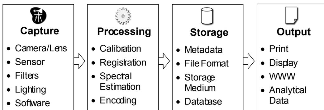
Figure 1: System components of spectral imaging system.
